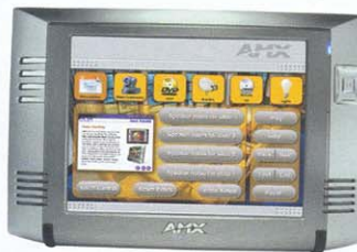
SMART Building touch-screen monitor
